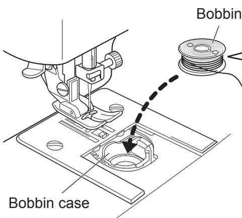
Thread unwinding direction
