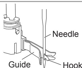
The hook is within the guide. The hook passes through the needle, catches the thread, then pulls the thread through the needle.
