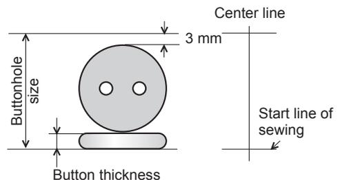
(Button diameter+button thickness+3mm)
