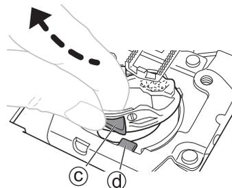
**4** Pull out the bobbin case in the direction of the arrow to remove it.
