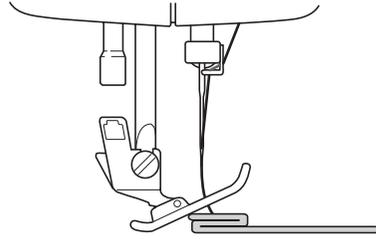
**Place fabric or thick paper of the same thickness as the fabric you wish to sew under the presser foot. This will enable smooth sewing.**
