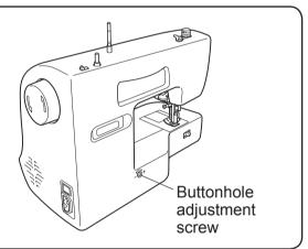
If the stitches are loose on the left side of the buttonhole, turn slightly in the "+" direction.
