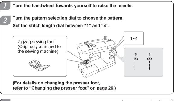
Position the fabric and lower the presser foot lever.
