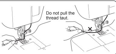
Lightly pull the upper thread with your left hand to pull up the lower thread.
