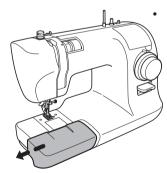
Pull out the extension table (accessory box) in the direction of the arrow.
